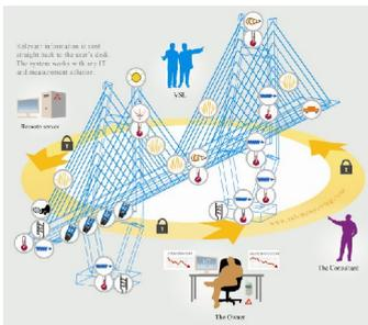
To guarantee the safety of users, large bridges have to be permanently monitored. VSL has developed a procedure for real-time surveillance of bridge reactions, using around 1,000 sensors from which information is immediately available on a secure extranet site.
