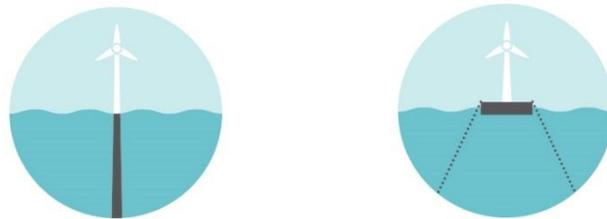
*Fixed-bottom offshore wind turbine Floating offshore wind turbine*
